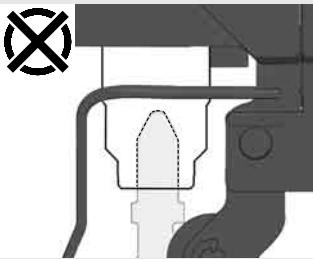
Press the saw blade into the Fixtec holder up to the stop.
